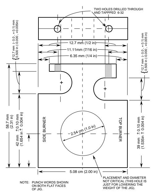
FIGURE 10. JIG FOR SETTING BURNERS AT PROPER DISTANCES FROM MATTRESS / FOUNDATION
