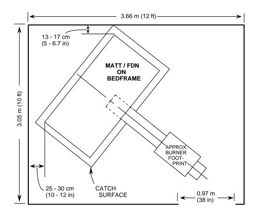
FIGURE 3. TEST ARRANGEMENT IN 3.05 m x 3.66 m (10 ft x 12 ft) ROOM; CONFIGURATION C.
