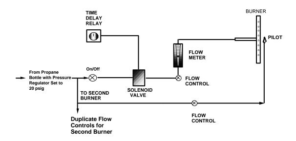
FIGURE 8. ELEMENTS OF PROPANE FLOW CONTROL FOR EACH BURNER
