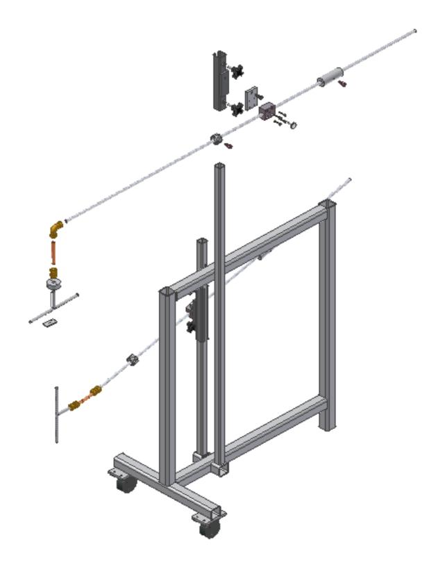
Figure 7. Burner Assembly Showing Arms and Pivots (Shoulder Screws) in Relation to Portable Frame Allowing Burner Height Adjustment.
