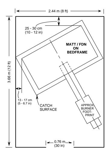
FIGURE 2 . TEST ARRANGEMENT IN 2.44 m x 3.66 m (8 ft x 12 ft) ROOM; CONFIGURATION B.
