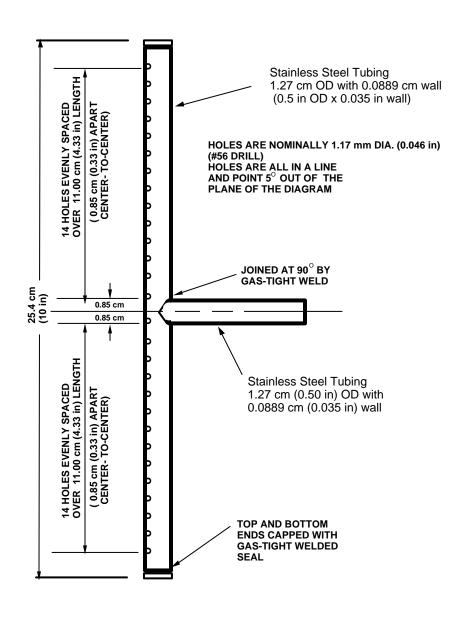
FIGURE 5. DETAILS OF VERTICAL BURNER HEAD.
