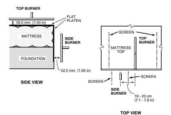
FIGURE 9. BURNER PLACEMENTS ON MATTRESS / FOUNDATION
