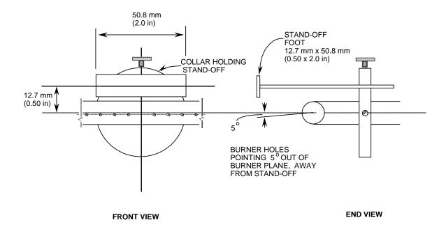
FIGURE 6. DETAILS OF BURNER STAND-OFF
