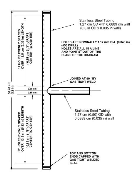
FIGURE 4. DETAILS OF HORIZONTAL BURNER HEAD.
